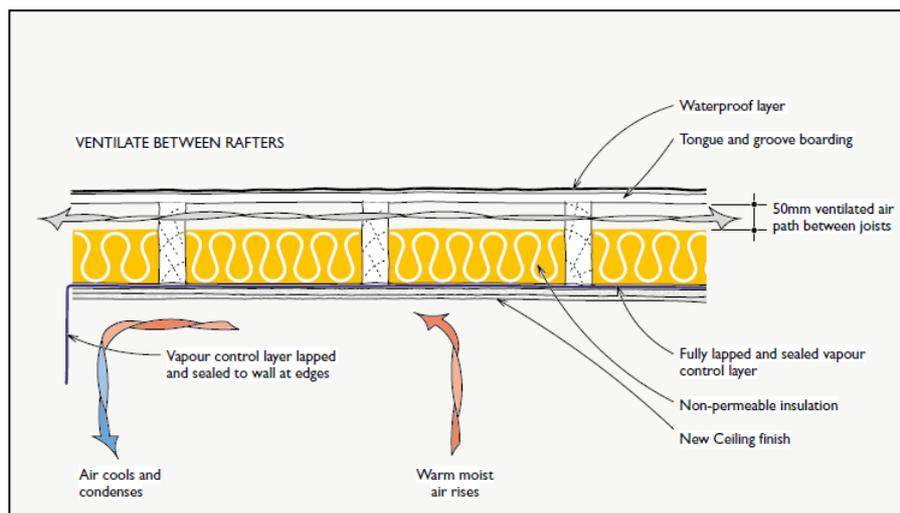
Fig 4. Ventilated cold deck using vapour permeable insulation
