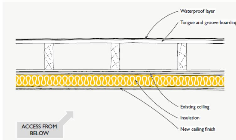
Fig 6. Insulation added below roof structure
