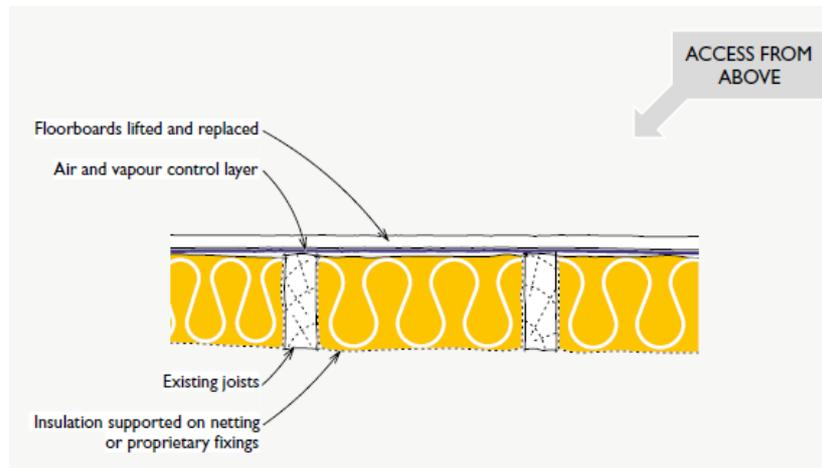
Fig 3. Fixing insulation from above floor
