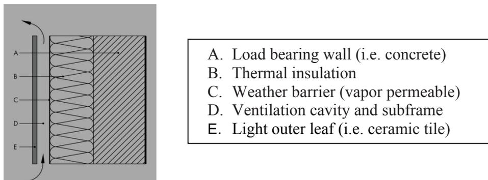
Fig 2. Scheme of a ventilated facade
