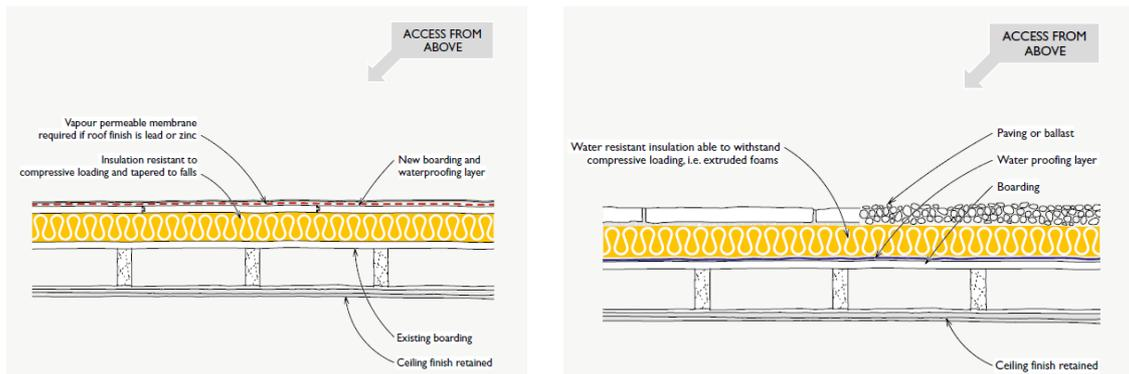
Fig 5. Warm deck system and Inverted system
